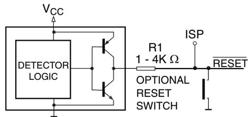
**Figure 7.** Detector with Open-drain Output
