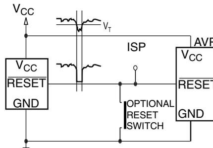
**Figure 12.** Integrated Reset Circuit with Adjustable Threshold Voltage
