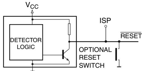
**Figure 8.** Alternative Location of Manual Reset Switch
