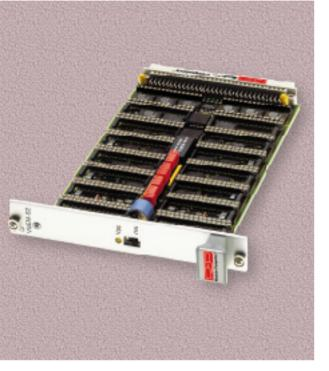
Typical applications can include hard disk replacement in harsh environments where adverse temperature and vibration make it unsuitable to use conventional spinning memory devices.
