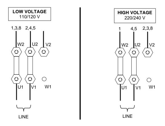
There are 6 wires from the motor housing numbered 1,2,3,4,5 and 8. Identify correct drawing above and connect the wires to terminals as shown.
