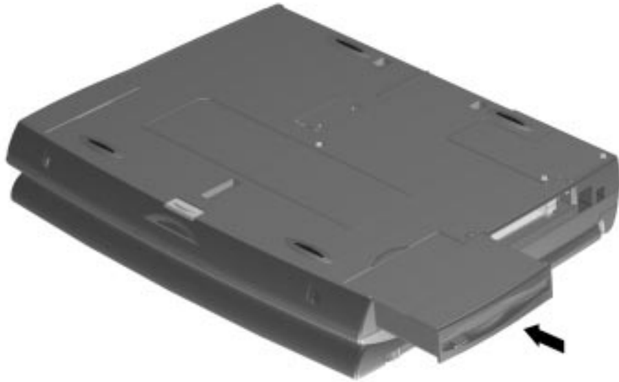
Figure 5-5. Installing the DualBay Device
