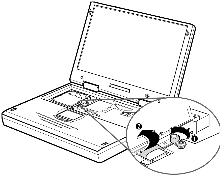
Figure 4-14. Removing the Hard Drive
