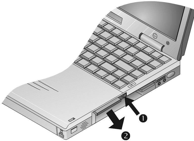
Figure 4-10. Removing the Internal Modem/Ethernet Combo Card
