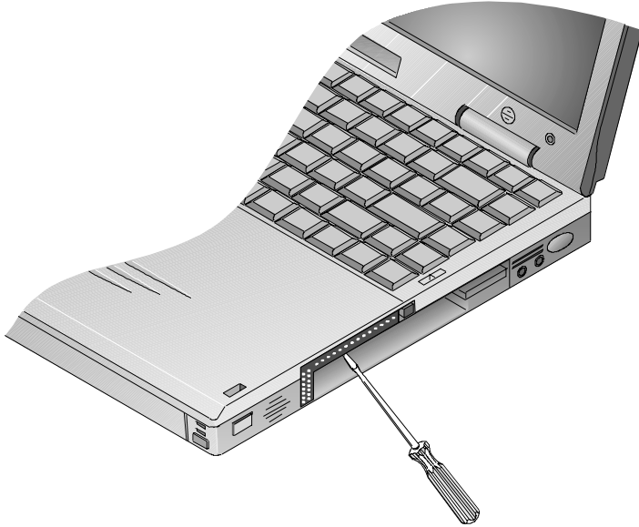
Figure 4-9. Removing the UMI Connector
