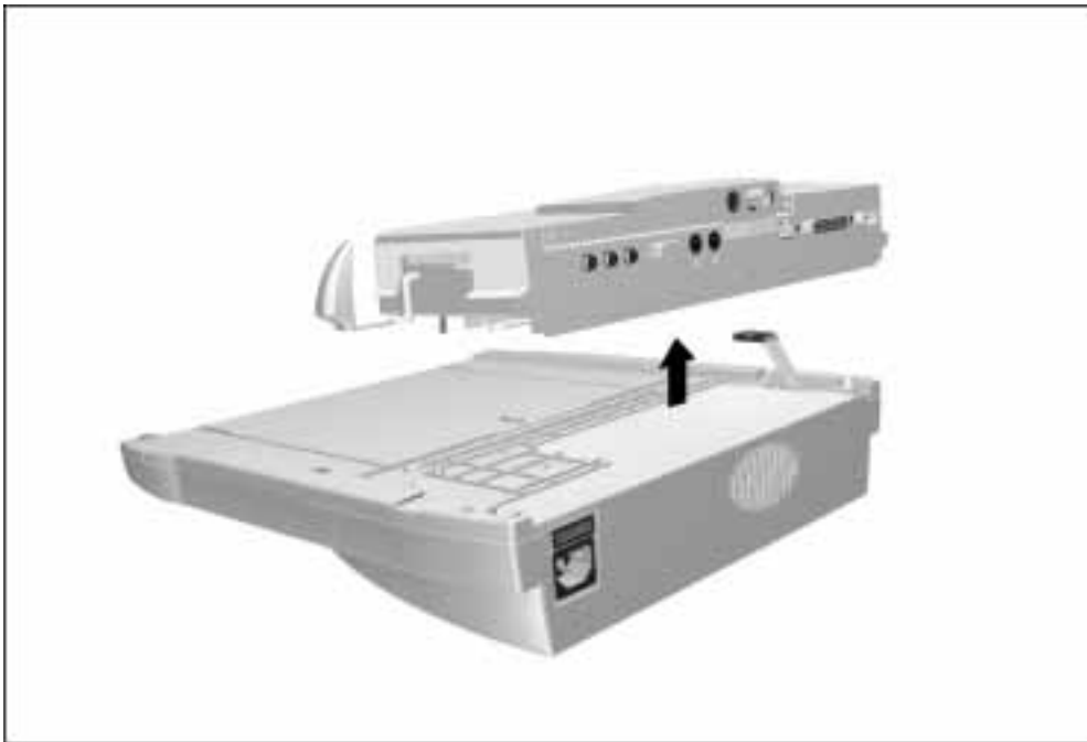
Figure 6-9. Removing the Module Assembly
