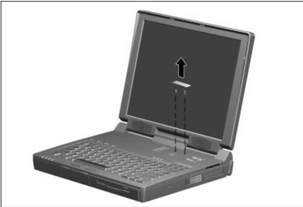
Figure 5-30. Removing the Keyboard Warning Label and Screws
