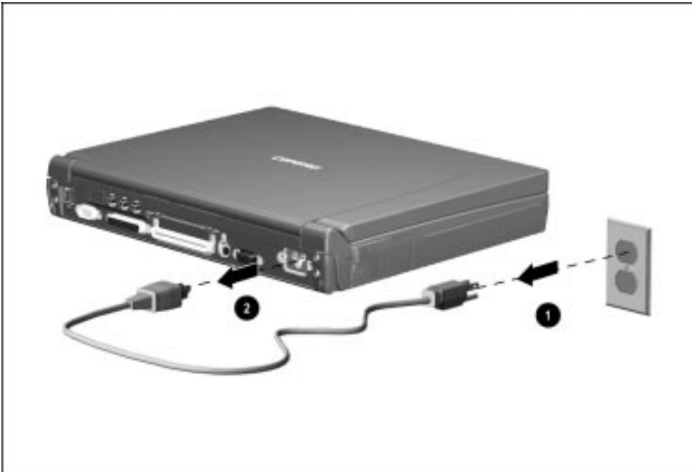
Figure 5-5. Disconnecting the Computer
