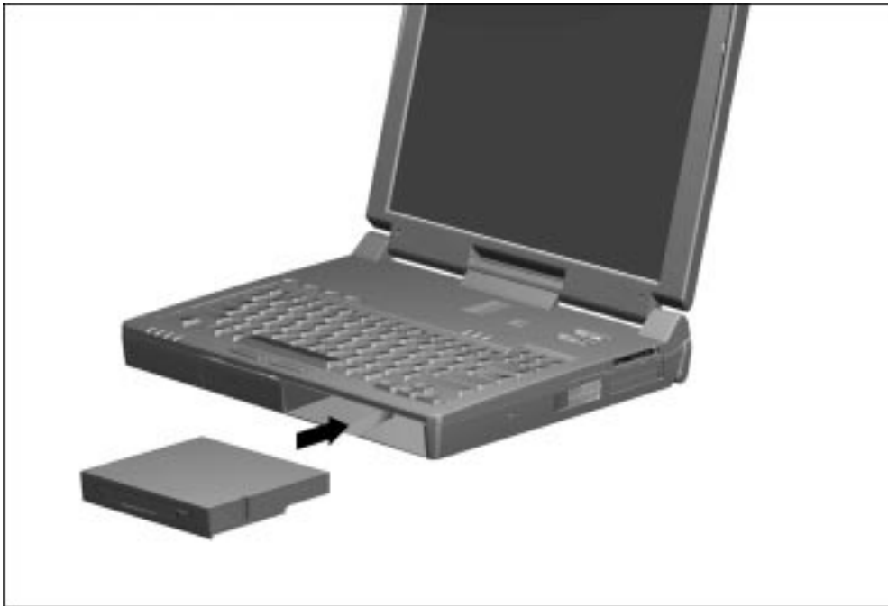
Figure 5-24. Inserting a Drive into the MultiBay
