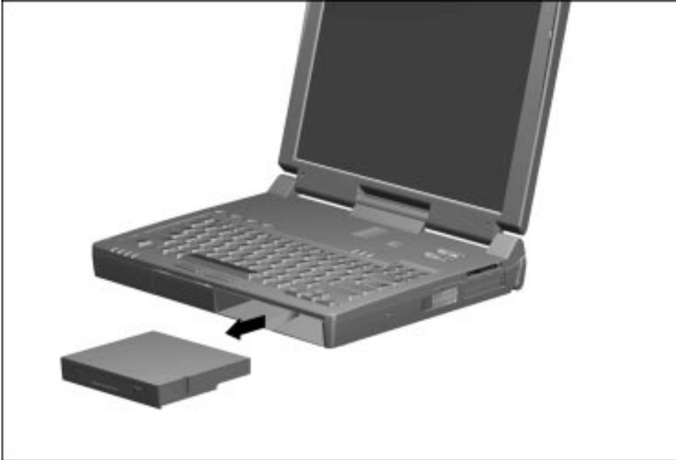
Figure 5-23. Removing a Drive from the MultiBay
