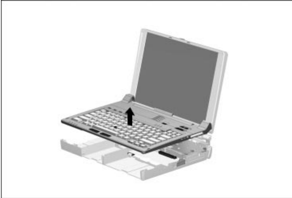
Figure 5-31. Removing the Keyboard Assembly
