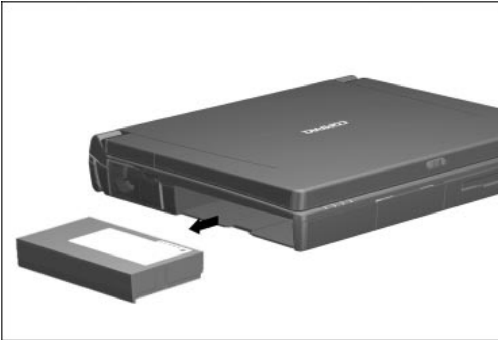
Figure 5-9. Removing a Battery Pack from the Battery Bay
