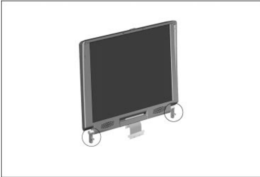
Figure 5-54. Proper Position of the Display Clutches
