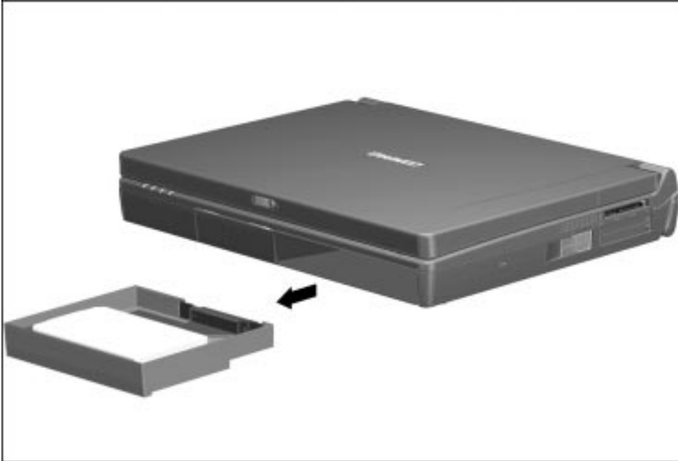
Figure 5-21. Removing the Hard Drive Assembly from the MultiBay
