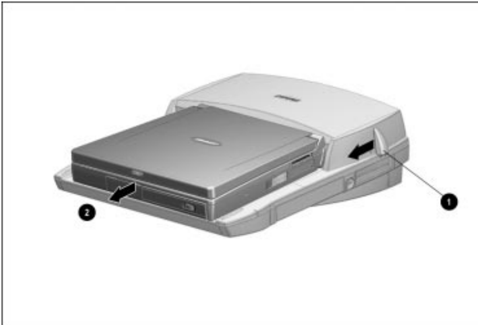
Figure 5-4. Undocking the Computer from the Armada MiniStation
