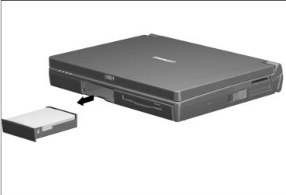
Figure 5-15. Removing a Hard Drive from the Hard Drive Bay
