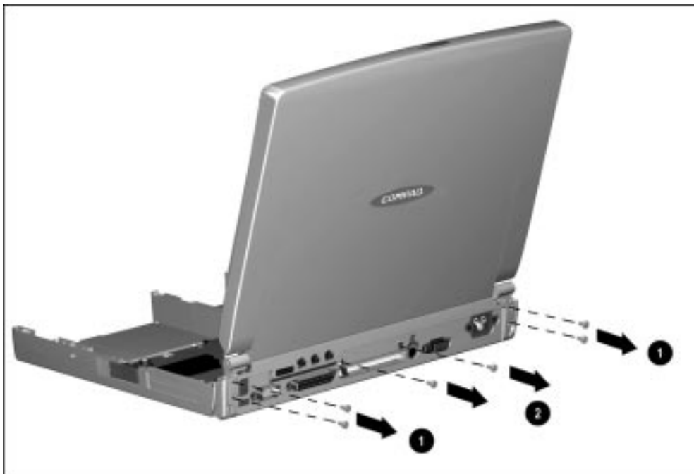
Figure 5-50. Removing the Display Assembly and Auxiliary Battery Assembly Screws
