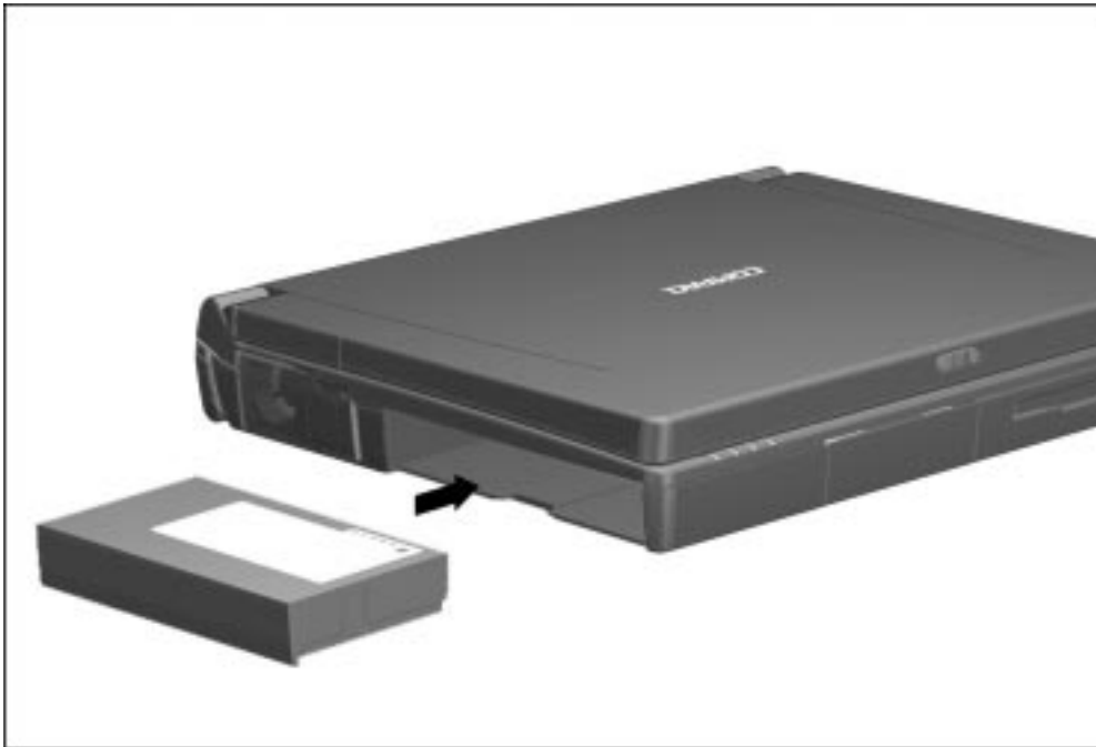
Figure 5-12. Inserting a Battery Pack into the Battery Bay
