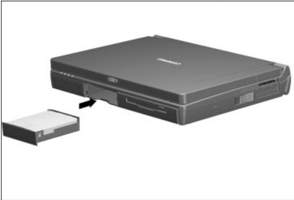
Figure 5-18. Inserting a Hard Drive into the Hard Drive Bay
