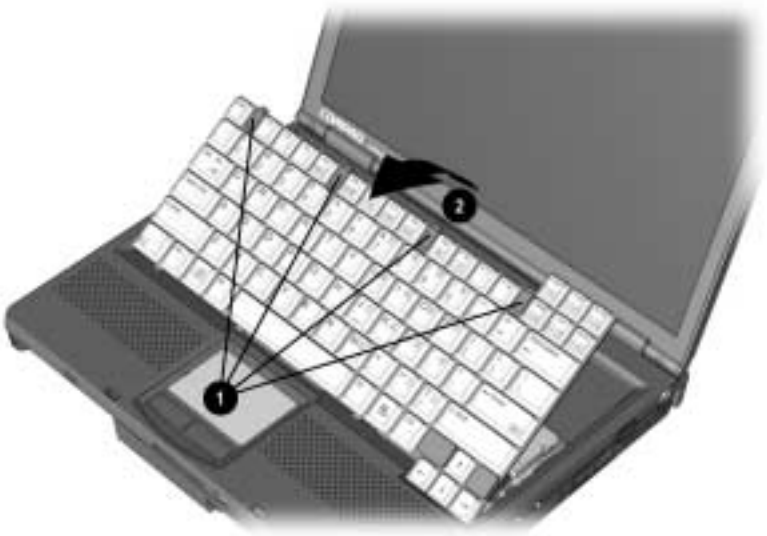
Figure 5-8. Releasing the Keyboard
