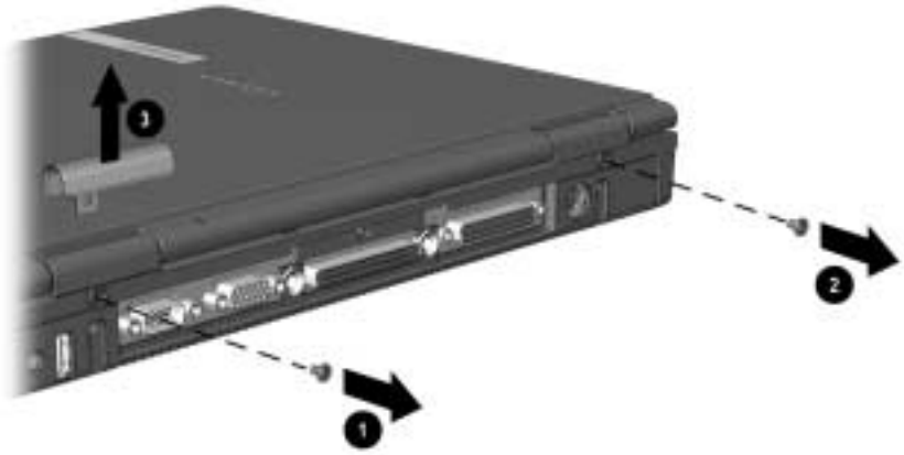
Figure 5-12. Removing the Switch and Hinge Cover Screws
