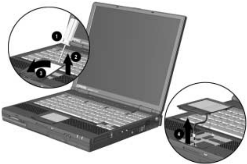
Figure 5-5. Removing the Touch Button
