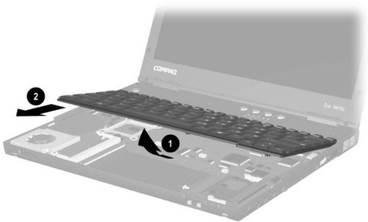
Figure 5-18. Releasing the Keyboard
