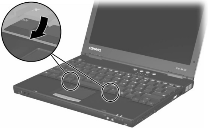
Figure 5-6. Releasing the Palm Rest
