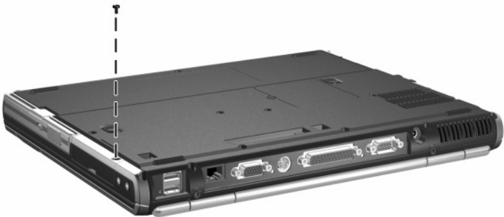
Torx T8M2.5x5.0 Screw Location
