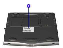
The Notebook serial number should be provided to Compaq whenever requesting information or ordering spare parts. The serial number 0 is located underneath the unit.
