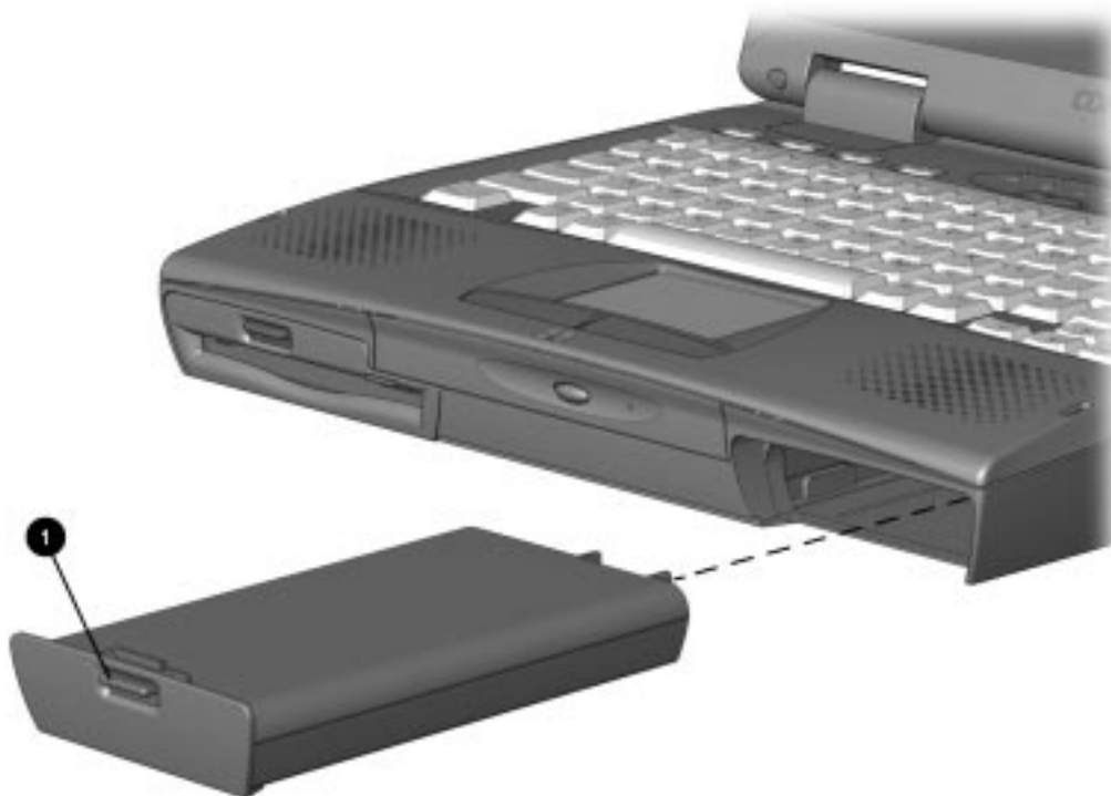
Figure 5-2. Removing the Battery Pack
