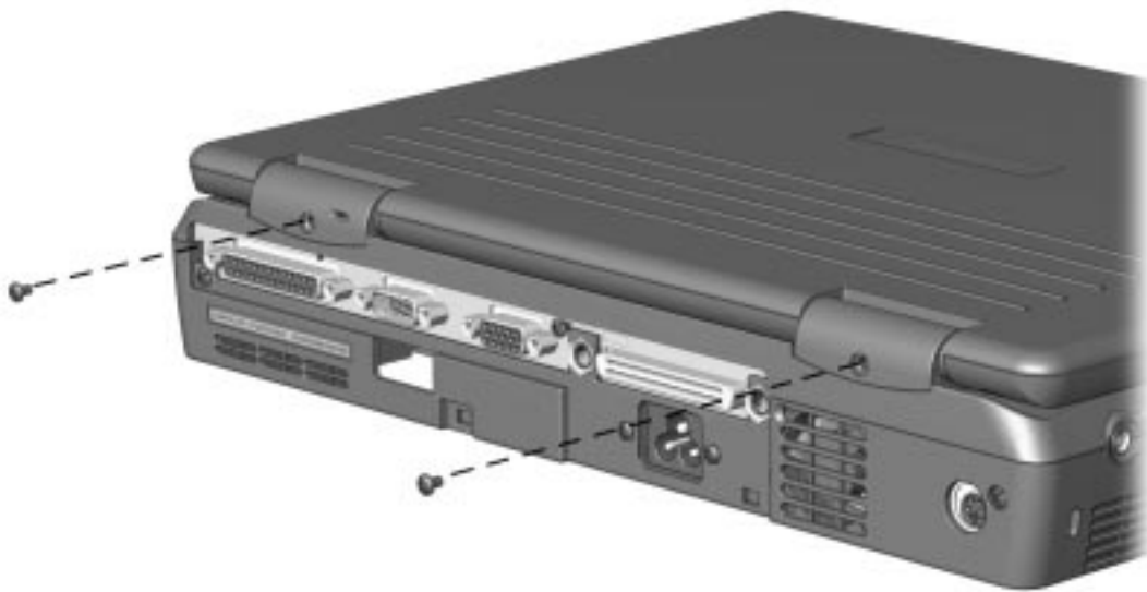
Figure 5-21. Removing the Hinge Cover Screws
