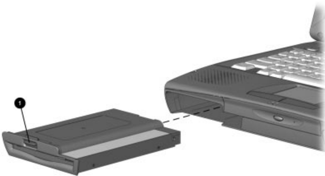
Figure 5-3. Removing the MultiBay Device
