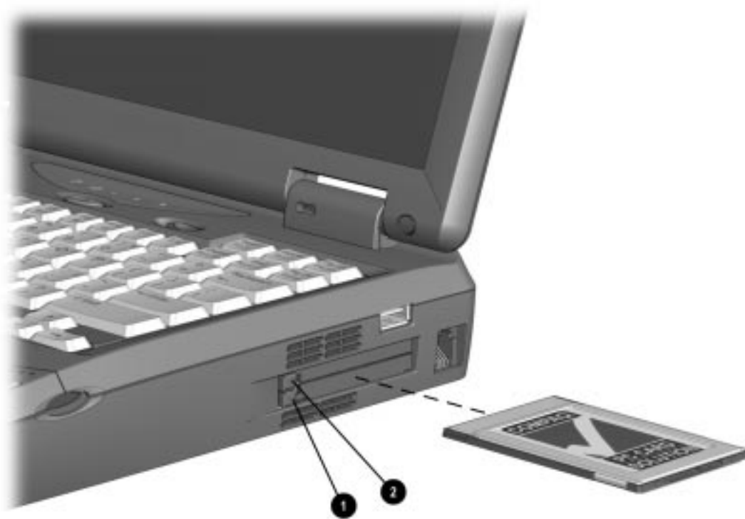
Figure 5-4. Removing the PC Card
