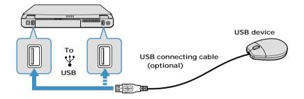
You can use an optional Sony USB mouse such as the PCGA-UMS1 series (optional) with this notebook. Since the USB mouse software driver is preinstalled in the notebook, you simply plug the USB mouse into the USB port to use it. One USB port supports one USB device.
