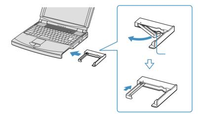
3 Manually lock the weight saver's Release lever.
