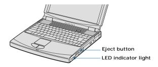
Do not push the eject button when the LED indicator is turned on. Otherwise, data may be lost.
