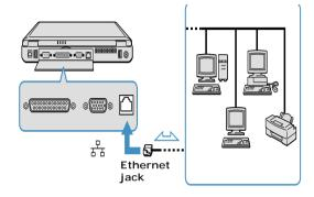
Warning: Only connect 10Base-T and 100Base-TX cables to the  $\frac{\Box}{\Box}$  Ethernet jack. Do not connect any other type of network cable or phone cable. Connecting cables other than those listed above may result in an electric current overload and could cause a malfunction, excessive heat, or fire in the port. To connect the unit to the network, contact your network administrator.
