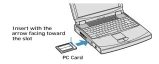
Do not force a PC Card into the slot as this may damage the connector pins.
