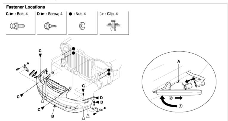
4. After removing the radiator grille (A), disconnect the cover (B) and rail (C).
