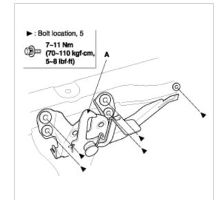
3. Disconnect the hood latch cable (A) remove the hood latch (B).
