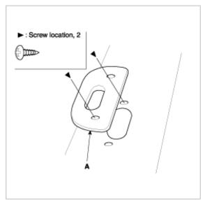
3. Remove the clips and fasteners, then remove the carpet (A). Put on gloves to protect your hands.
