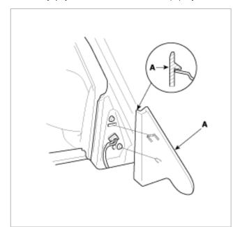
3. Disconnect the connector (A), then remove the mirror mounting bolts while supporting the mirror (B).
