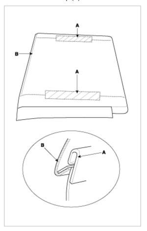
4. Disconnect the headrest guide (A), after raising the rear seat back frame (B).
