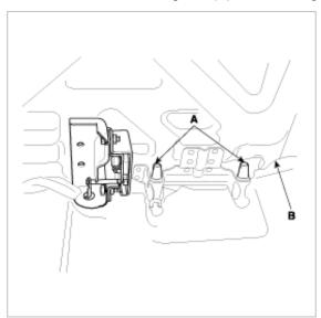
5. Pull back the edge of the seat-back cover (A) all the way around, and release the clips (B), then remove the seat-back cover.
