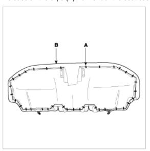
3. Pull back the edge of the seat cushion cover all the way around, and release the clips (A), then remove the seat cushion cover. On a leather seat cover (B), there are no fasteners.
