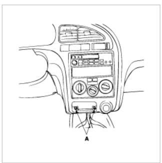
5. Disconnect the connectors from the instrument facia panel.
