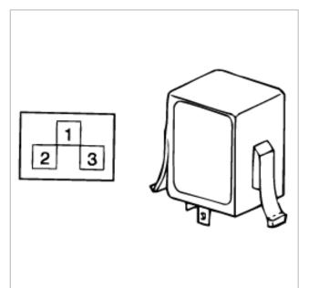
3. Connect the two turn signal lamps in parallel to terminal 1. Check that the bulbs turn on and off.
