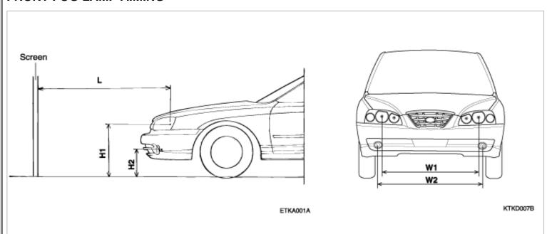
H1 : Height between the head lamp bulb(low beam) center and ground
