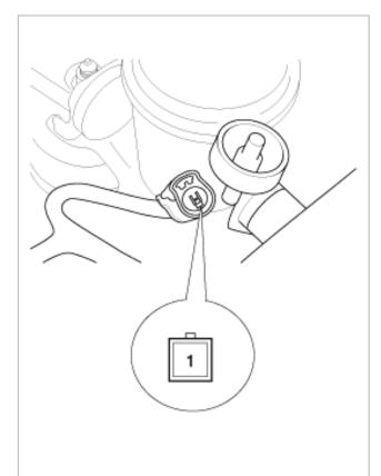
2. Check for continuity between the terminal and ground according to the table.
