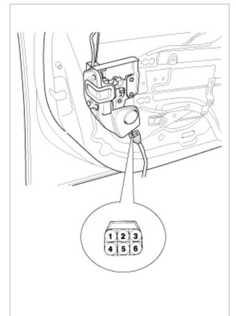
3. Check for continuity between the terminals in each switch position according to the table.
