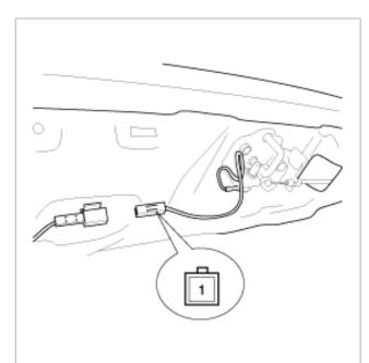
4. Check for continuity between the terminal and body while pushing the rod.
