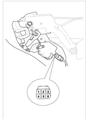
3. Check for continuity between the terminals in each switch position according to the table.
