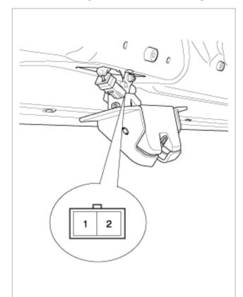
3. Check for continuity between the terminals according to the table.
