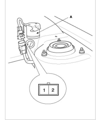
2. Test the siren by connecting battery power to the terminal 1 and ground the terminal 2. The siren should make a sound. If the siren fails to make a sound replace it.
