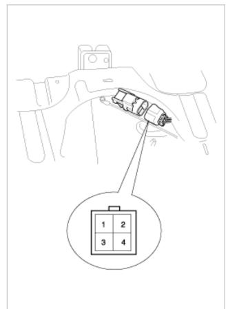
3. Check for continuity between the terminal in each switch position according to the table.
