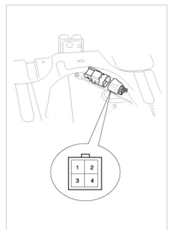
3. Check actuator operation by connecting power and ground according to the table. To prevent damage to the actuator, apply battery voltage only momentarily.
