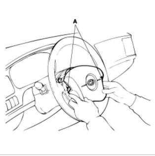
3. Remove the steering wheel after removing a nut(A).
