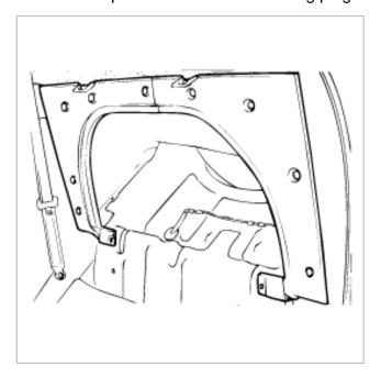
3. Remove the bolts(A) and plugs(B) from the rear package tray trim.
