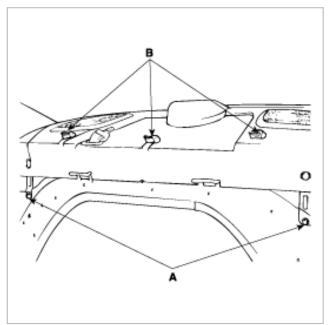
4. Remove the rear seat belt lower mounting bolt(A).
