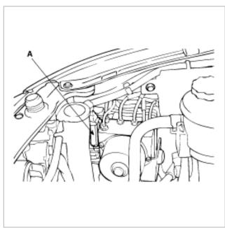
2. Disconnect the brake tubes from the HECU.
