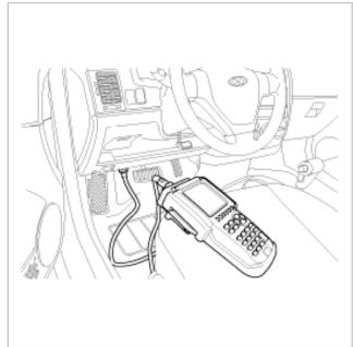
4. Select and operate according to the instructions on the hi-scan (Pro) screen.
