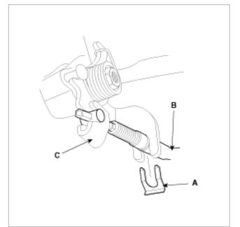
2. Disconnect the parking brake cable (B) from the lever (C).
