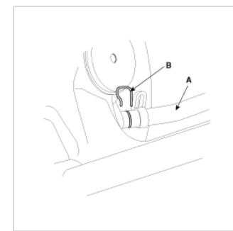
3. Remove the parking brake cable (A) from the backing plate (B).
