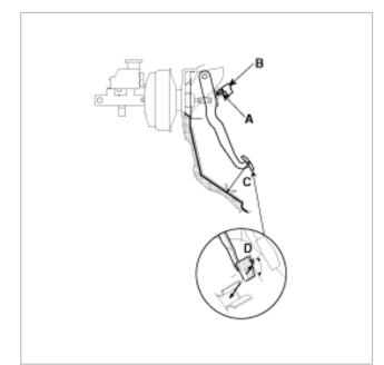
3.Loosen the pushrod locknut (A), and screw the pushrod in or out with pliers until the standard pedal height from the floor is reached. After adjustment, tighten the locknut firmly. Do not adjust the pedal height with the pushrod depressed.
