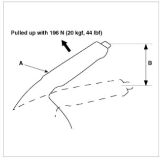
2. Adjust the parking brake if the lever clicks are out of specification.
