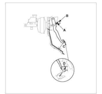
3. Loosen the pushrod locknut (A), and screw the pushrod in or out with pliers until the standard pedal height from the floor is reached. After adjustment, tighten the locknut firmly. Do not adjust the pedal height with the pushrod depressed.
