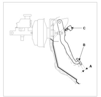
2. If the pedal free play is out of specification, adjust the brake switch (C). If the pedal free play is insufficient, it may result in brake drag.
