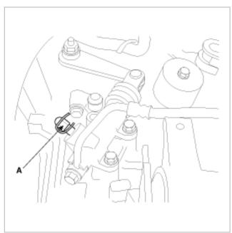
2. Remove clevis pin (A), split pin (cotter pin) (C) and washer (B).
