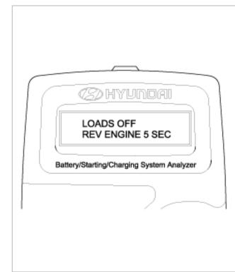
5. The MICRO 570 analyzer charging system output at idle for comparision to other readings.
