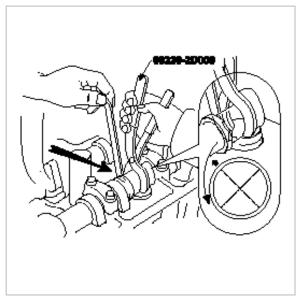
C.Remove the adjusting shim with a small screw driver and magnet.
