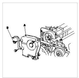
4. Turn the crankshaft pulley, and align its groove with timing mark "T" of the timing belt cover.
