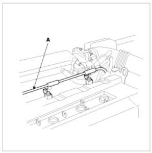
D.Loosen the cylinder head cover bolts and then remove the cover and gasket.
