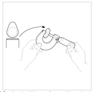
E.Caculate the thickness of a new shim so that the valve clearance comes within the specificified value.
