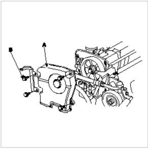
A. Loosen the upper timing cover bolts and then remove the cover.
