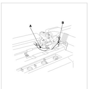
C.Disconnect the accelerater cable (A) from the cylinder head cover.
