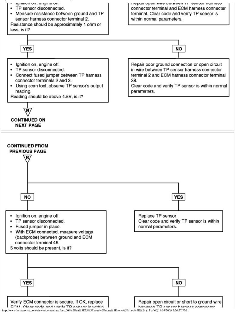
Verify ECM connector is secure. If OK, replace ECM. Clear code and verify TP sensor is within normal parameters. Repair open circuit or short to ground wire between TP sensor harness connector terminal 1 and ECM harness connector terminal 32.
