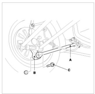
2. Remove the bolt (C) fixing the rear suspension arm (A) to the rear carrier (B).
