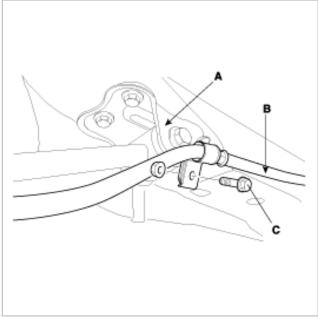
2. Remove the trailing arm mounting bolts(A,B) and the trailing arm bracket mounting bolts(C,D,E).
