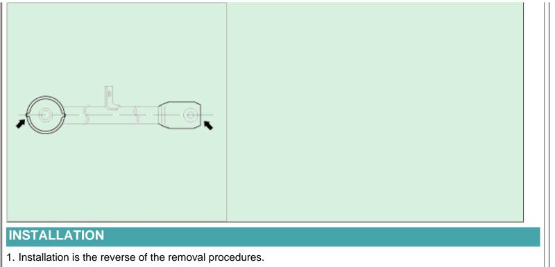
2. Fully tighten the trailing arm mounting bolts to the specified torque under the unloaded vehicle on the ground.
